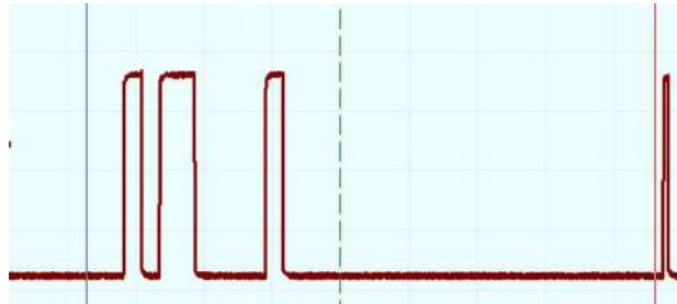
Glitches in clock or power lines
